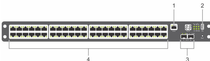
Figure 1. N2048 Series with 48 10/100/1000BASE-T Ports
